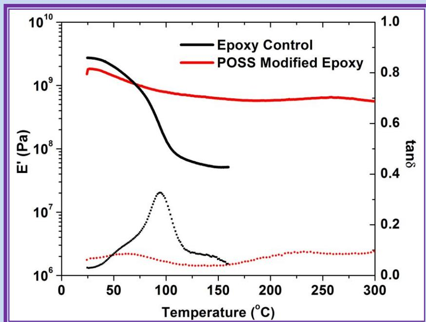
modified composite materials have much higher use temperatures and can tolerate very high temperature thermal spikes. POSS® epoxies also have excellent solvent resistance making them suited to medical and electronic applications.
