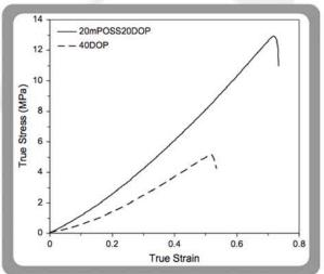
Increasing MA0735 concentration leads to a increase in the tensile strength of the plasticized PVC
